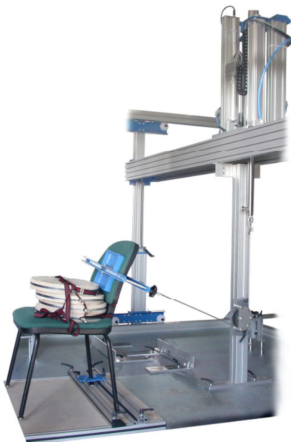
Installation set tilting and drop test for universal test fields order no.: 40-910-081
