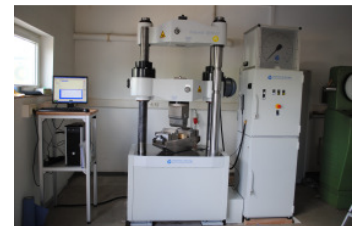
The universal testing machine Inspekt 1000-H performing a bending test on a welded specimen with a nominal thickness of 50 mm:
