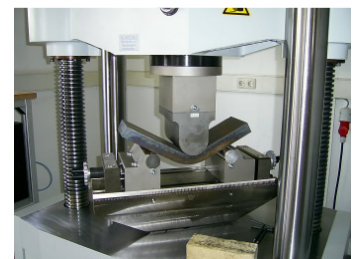
The universal testing machine Inspekt 1000-H performing a bending test on a welded specimen with a nominal thickness of 50 mm:
