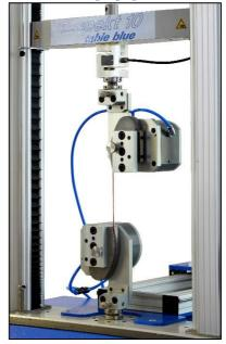
This grip is among others suitable for tensile tests on wires up to 4 mm thickness. The clamping force can be reduced by the bollard grip design. This decreases the risk of fractures at the grips significantly.
