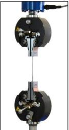
The long design of the clamping jaws allows a soft leading of the clamping force into the specimen, enhancing the tensile test by reducing the stress concentration at the end of the clamping area. It is known that specimen fracture may occur at the clamping jaw, if the cross sectional area of the free length and the clamped specimen is equal. Exactly this effect is prevented by the special jaw design.
