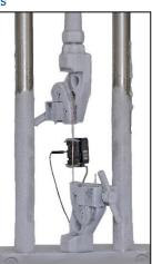
The enlacement clamping device for wires and tapes is designed for tensile tests with specimens up to a maximum load of 1kN. It is suitable for tests in liquid nitrogen down to -196°C.
