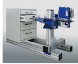
This furniture test rig conducts fatigue tests on drawers, drawer guides, and functional fittings.
