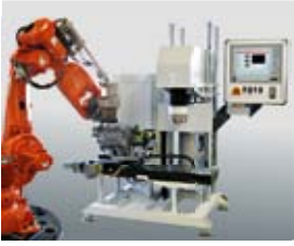
This automated hardness test center works in a foundry. It tests the Brinell hardness of engine blocks – hundreds a day.
