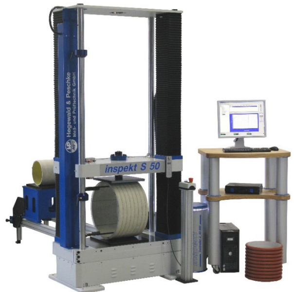
Compression testing machine 50 kN for pipes up to 1500 mm Item no. 10-003-906
