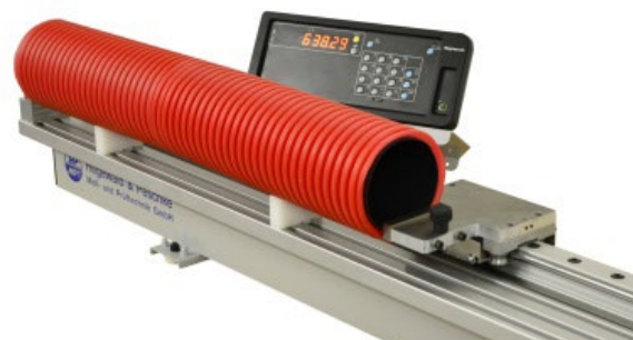
Length measurement on plastic pipes
