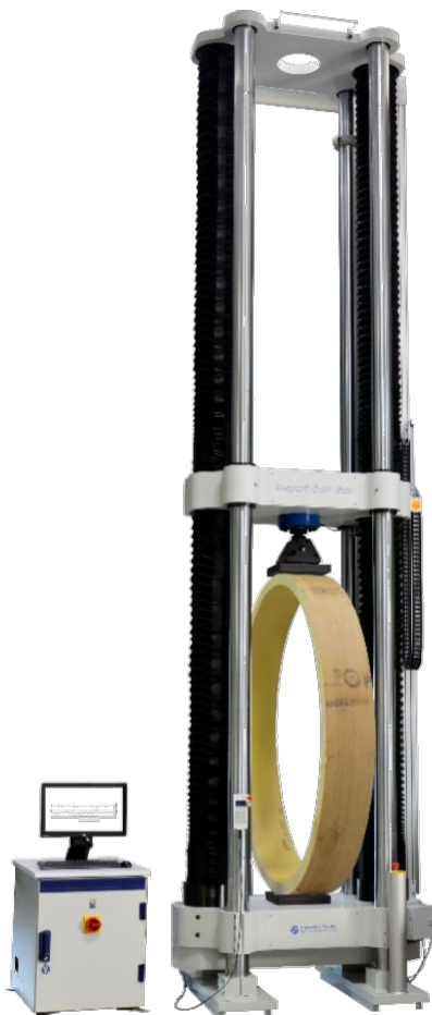
Testing machine 600 kN for GRP pipes with pipe diameters up to 4200 mm Item no. 10-003-806
