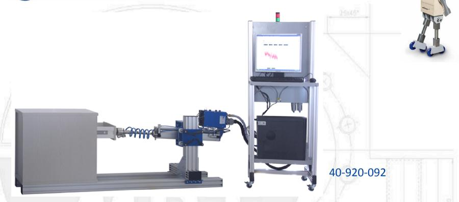
The pneumatic test axis is suited for long term loading, life cycle testing and fatigue testing on drawers, drawer components and sides e.g. in acc. to EN 15338, EN 1727 and DIN 68898.
