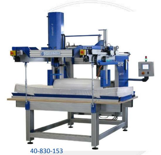
The automated test station combines the hardness and roller application in acc. to EN1957. Thus the mattress does not need to be transported during the test manipulating tests results, but after placing the mattress at the test fixture the operator only needs to choose test program (can be customized) and the complete test runs automated. All hardness results will be recorded in reference to the cycle number and can be evaluated per mattress. A statistic evaluation is available.
