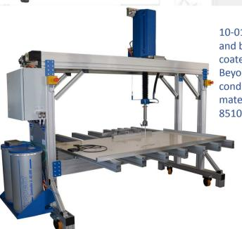
10-012-050 Testing of adhesion and bonding strength between the coated surface and the rigid carrier. Beyond a 90°-peel test can be conducted at the composite material e.g. acc. to DIN EN ISO 8510-1; exemplary solar module
