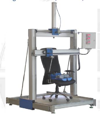
40-910-010: measurement device e.g. for distance measurement of seat depth, seat and arm rest, arm rest to arm rest.
