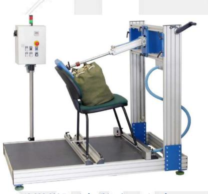
40-930-080 Test rig for tilting drop testing of fourfeeter indoor and office chair as well as outdoor furniture stool and cantilever chair (freeswinger chair) in acc. to DIN 68878.
