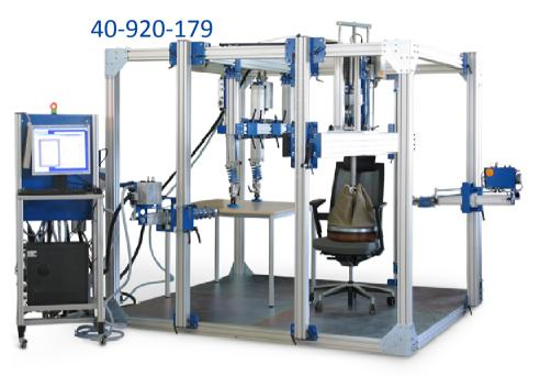
Universal test rigs with a static optimized and solid test frame and strong galvanized base plates with a thread pattern for easy and flexible fixation of specimen.
