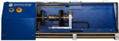
41-031-50x Torsion test stand T200, e.g. for twist testing at wire in acc. to DIN ISO 7800 and ASTM A938 as well as for transition twist testing at wires in acc. to DIN ISO 9649
