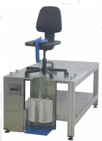
40-910-090 Stability test on chair and seating furniture acc. to EN 1022, EN 1729, EN 581-2-3, EN 1335, DIN 68878 and BIFMA X 5.1
