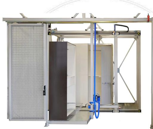
Combined test rig for revolving and sliding doors as well as for drawer
