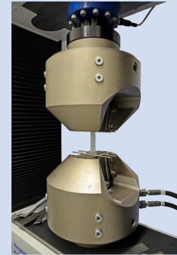
Special 250 kN hydraulic wedge type grip – body over wedge
