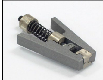
Thread grip for tensile tests at thin threads, yarns or twines
