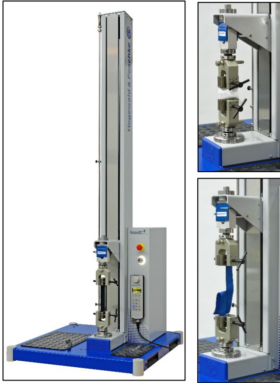
Universal testing machine Inspekt solo 2.5kN with vice grip
