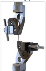
The enlacement clamping device for wires and tapes is designed for tensile tests with specimens up to a maximum load of 1kN. It is suitable for tests in liquid nitrogen down to -196°C.
