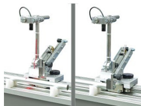
Combi mobile stop with line laser (left: optical measurement of sample center / right: mechanical probing at the sample end)
