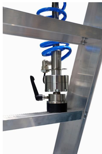
Fig. 1: Load pad on a pneumatic test axis during continuous loading test according to EN 131
