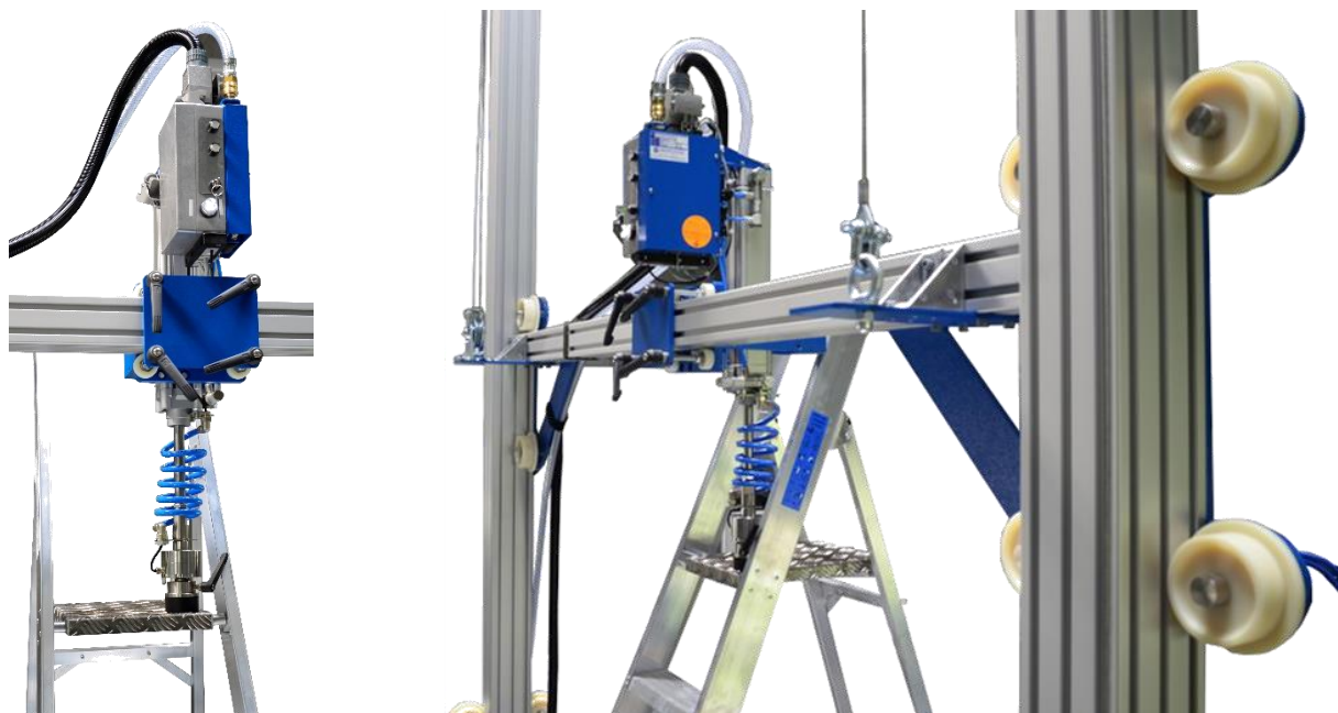
Fig. 3: Test cylinder, front view (left) and view on cross profile (right)
