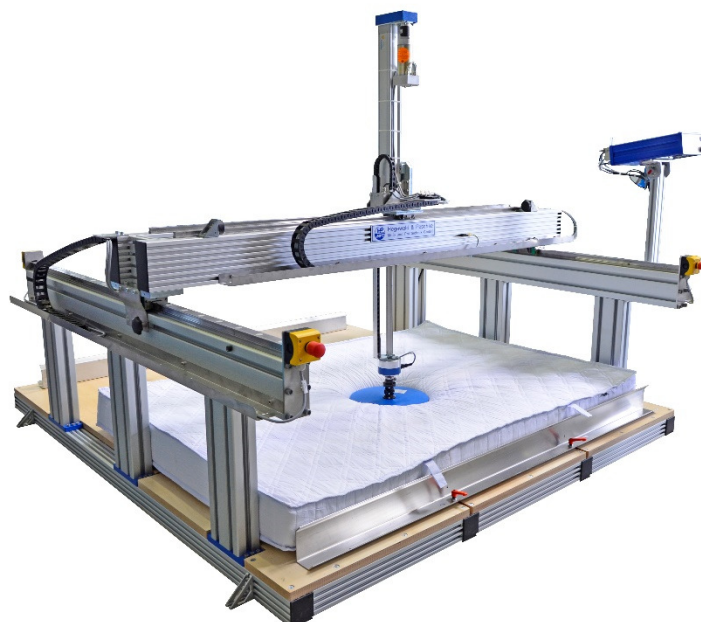
Single test stand for the hardness measurement on mattresses, spring cores and (box spring) beds according to EN 1957 (Art.-No.: 40-830-158)
