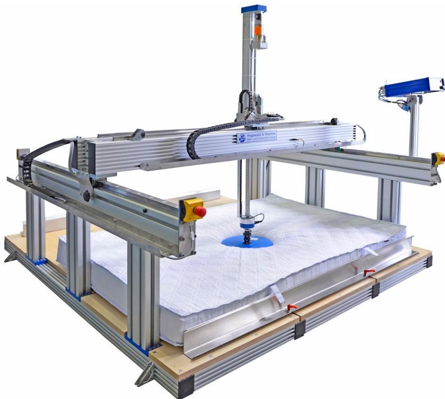
Single test stand for the hardness measurement on mattresses, spring cores and (box spring) beds according to EN 1957 (Art.-No.: 40-830-162)
