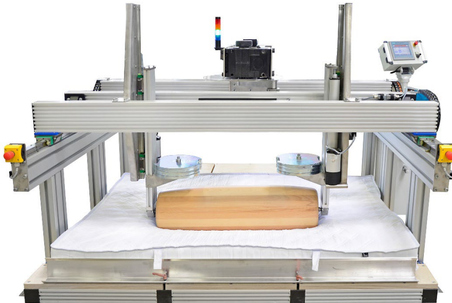
Single test stand for durability tests on mattresses, spring cores and (box spring) beds according to EN 1957 (Art.-No.: 40-830-164)
