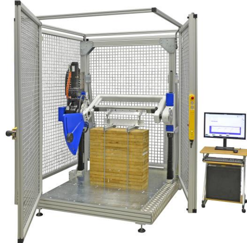
Test rig for fitting tests on hinges and flap mechanisms (41-041-425)
