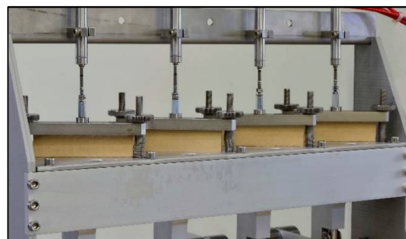
Fig. 2: detailed view pressure pieces and measuring sensors
