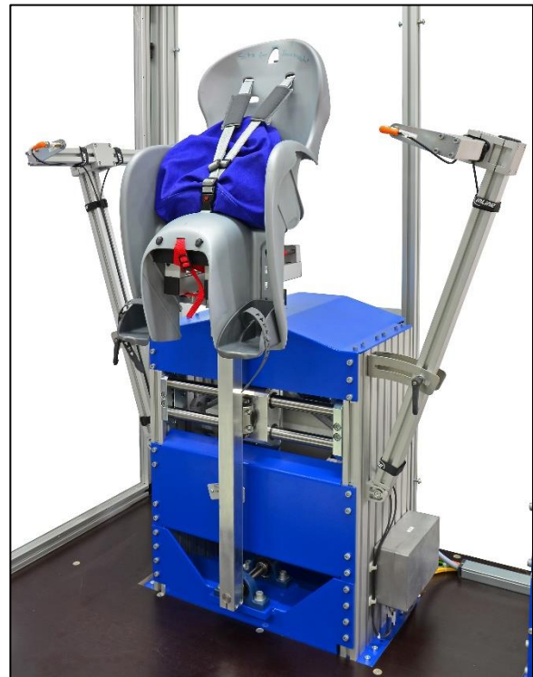
Fig. 1: Testing device for lateral and transverse stiffness testing
