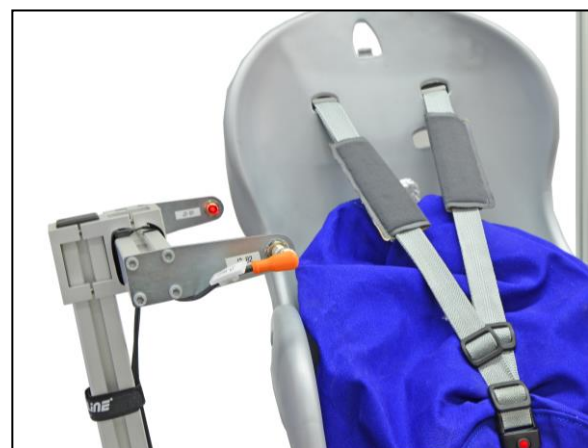
Fig. 2: Light barriers for monitoring the deflection
