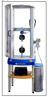
Wedge type grip with clamping jaw holders for the testing of round and flat wires as well as other semi-finshed specimens
