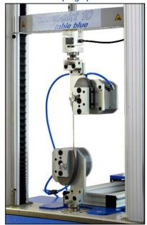
This grip is among others suitable for tensile tests on wires up to 4mm thickness. The clamping force can be reduced by the bollard grip design. This decreases the risk of fractures at the grips significantly.
