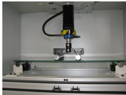
4-point bending test according to DIN EN 1288-3
