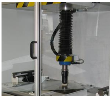
Static puncture test according to ISO 614
