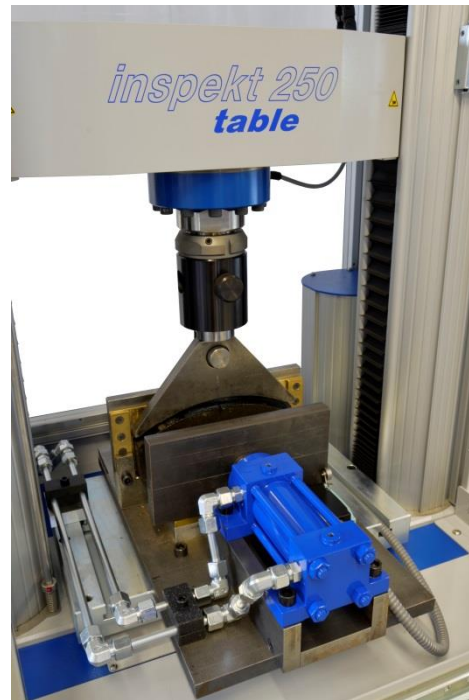
Fig. 1: Shear test on a brake shoe
