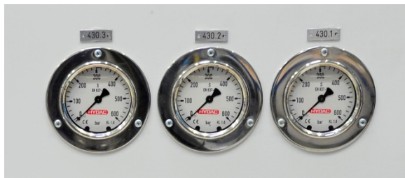
Fig. 1: Analogue service display for clamping pressure top/bottom and system pressure
