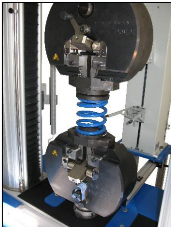
Test system wedge type grip with adapted compression plates for spring testing
