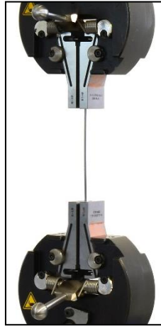
Test system Wedge type grip with extended clamping jaws (item no.: 14-096-590 or 14-096-591) for clamping of wires
