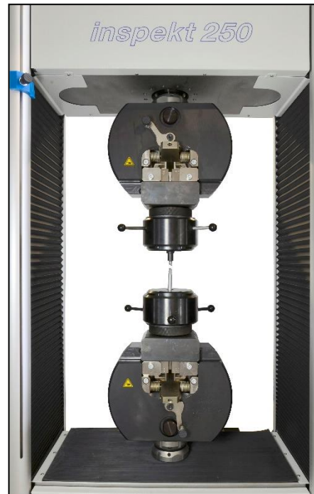
Test system wedge type grip with adapted specimen holder for the testing of threads
