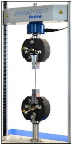
Test system Wedge type grip with extended clamping jaws (item no.: 14-096-590 or 14-096-591) for clamping of wires
