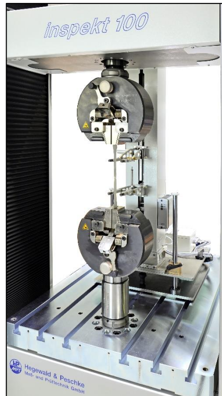
Test system wedge type grip with long distance extensometer MFN-A
