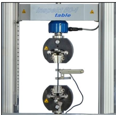
Test system wedge type grip with clip-on extensometer MFA-25
