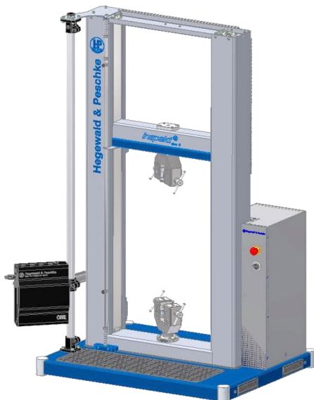
Mounting video extensometer ONE at inspekt duo (15-008-230)
