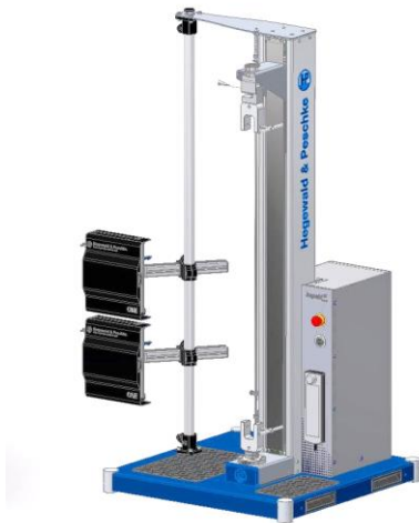
Mounting video extensometer ONE at inspekt solo (15-008-130) (with multi-camera system)
