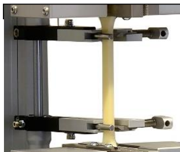
Fig. 1: Measuring arms on a plastic specimen C-type (standard)
