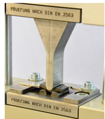
3-point miniature bending device for GRP/CFRP specimens acc. to DIN EN 2563
