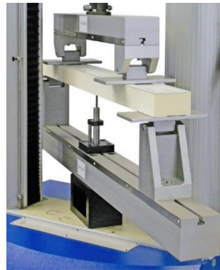
4-point bending test on ceramic high-performance materials according to EN 843-2 (method A)
