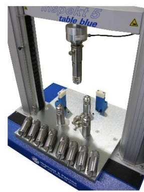
3-point miniature bending device for GRP/CFRP specimens acc. to DIN EN 2563
