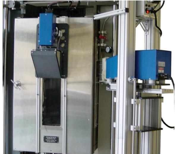
Fig. 4: Strain measurement on metals with a parallel scanner P-100 in a climatic chamber up to 650°C with vacuum channel
