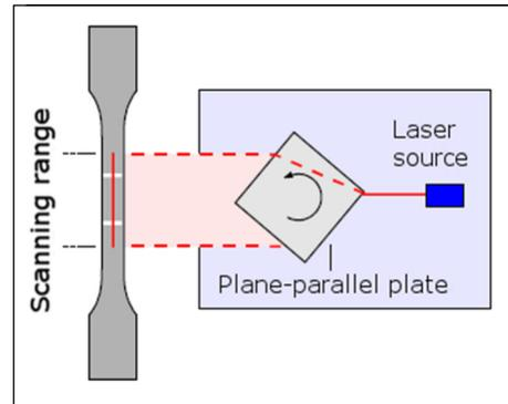
Fig. 1: Operating principle of parallel scanner
