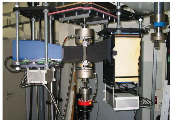
Fig. 5: Measurement of longitudinal and lateral strain with foam tunnel to avoid air turbulence
