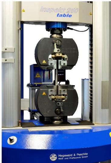
Fig. 3: Application P-50 with universal testing machine inspekt table 250kN for metal tensile test
