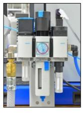
Operation of the grips via manual operation of the testing machine - Stepless adjustment of the main pressure possible in the testing software (item no. 14-005-330)
