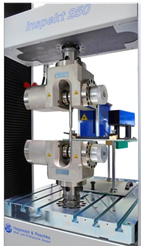
Fig. 6: SWS-300 for metal tensile test
