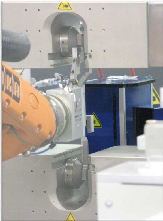
Fig. 4: Use of the SWS-300 in automated test system for metal tensile tests
