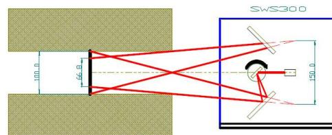
Fig. 2: Operating principle SWS-300 for short specimens
