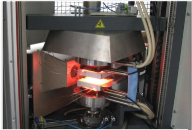
Fig. 5: Use of a vacuum tube for cyclic high-temperature strain measurement on insulation material for catalyst blocks
