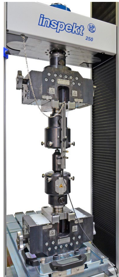
Coupling of the specimen holder to the screw type wedge action grip
