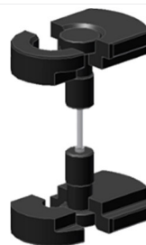
Screw testing with insertion plates and spherical inlay nuts
