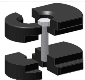
Screw testing with insertion plates and inlay nuts
