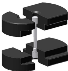
Wedge loading of screws with insertion plates and inlay nuts
