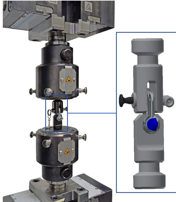
Coupling of the specimen holder to the screw type wedge action grip
