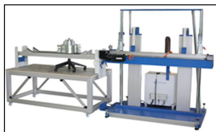
Fig. 1: Threshold test for rollers
